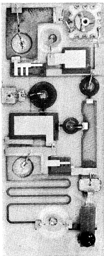
Fig. 2. Photograph of the thin film tunnel diode mixer.
